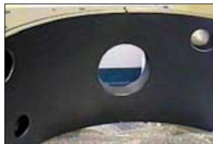
*Fig. 3 — UHP silicon coating (99.999 %) on internal surface of a process chamber. The coating is uniform and micro-conformal, with a clean and shining surface.*
