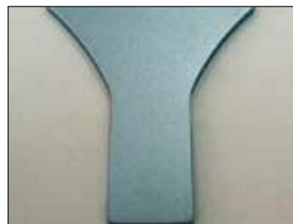
*Fig. 2 — An aluminum alloy 6061 part coated with ultra high purity silicon (99.999%). The coating thickness is about 25 μm.*
