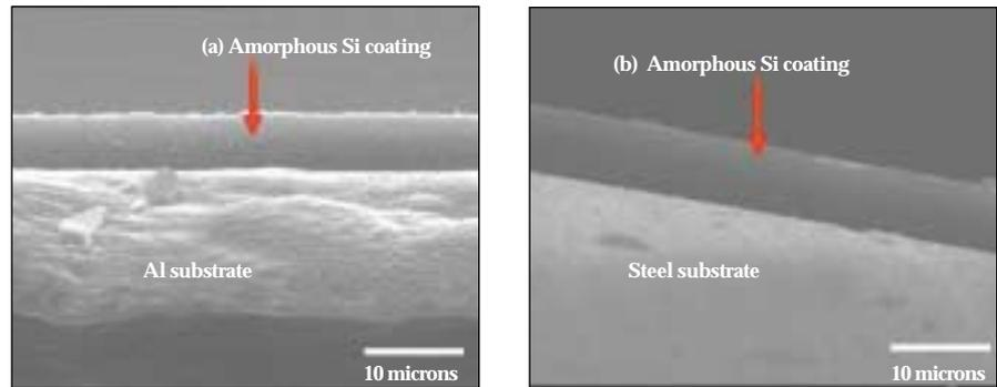
Fig. 1 — Cross-sectional SEM micrograph of ultra high pure silicon coating on (a) aluminum foil, and (b) steel blade. The coating is amorphous, microscopically homogeneous, and featureless.
