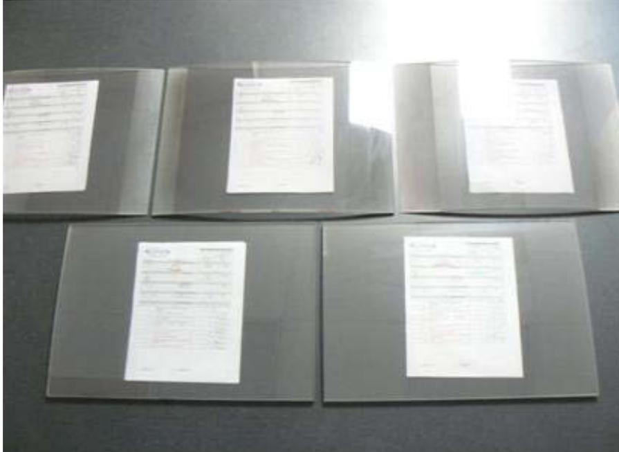
Figure 6: Cylindrically curved ALON<sup>®</sup> segments for Side Window for Automotive Application.
