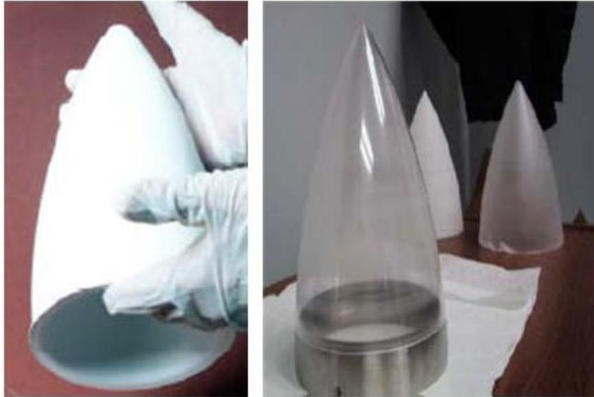
Figure 4. Tangent Ogive green body and finished domes.
