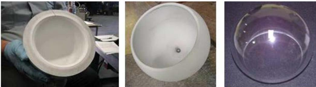
Figure 5. Hyper-hemispherical ALON<sup>®</sup> green bodies and finished dome.
