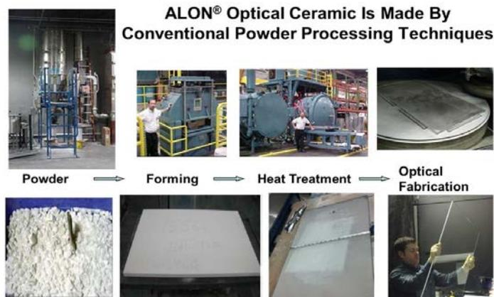
Figure 1. Schematic of process for producing ALON<sup>®</sup> Optical Ceramic.
