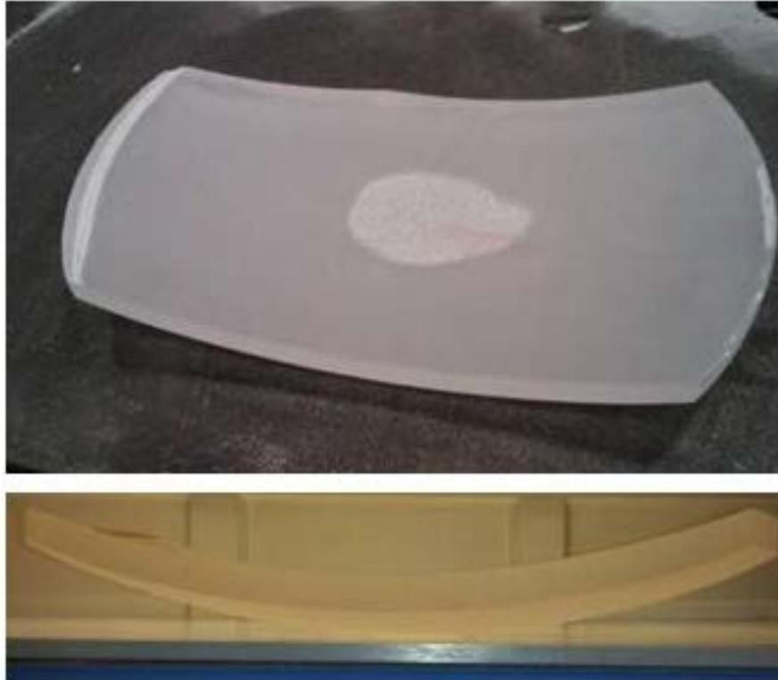
Figure 9. Photograph of conformal ALON® blank produced for sensor application. Top view (top) and Side View (bottom).
