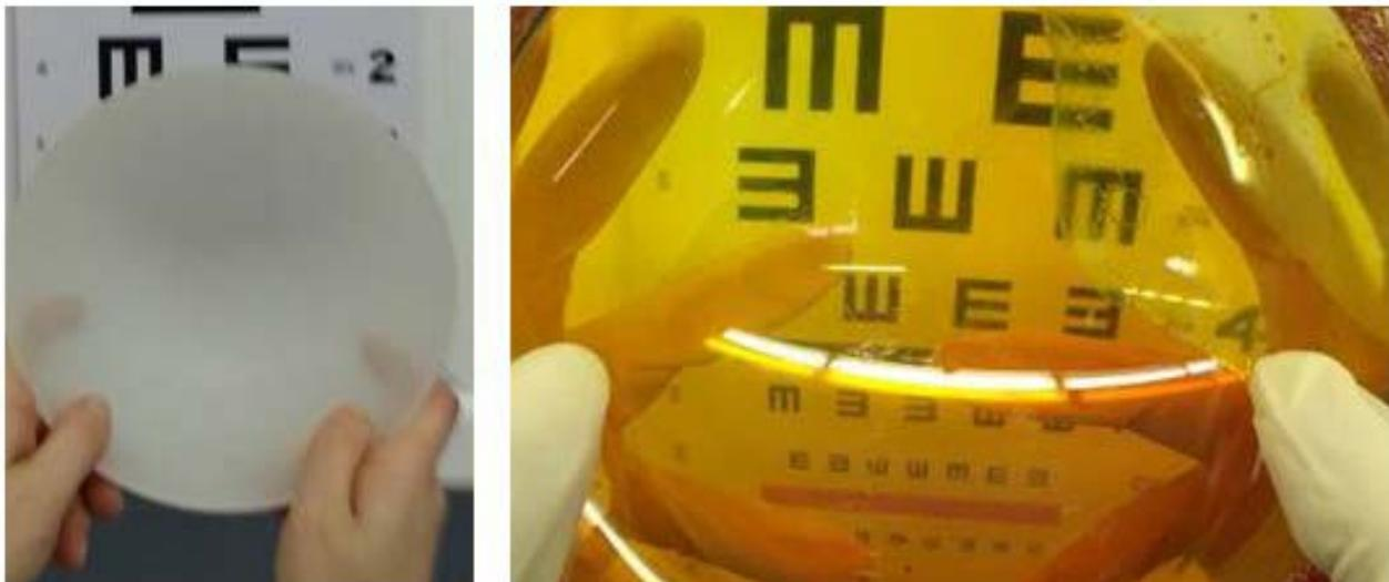
Figure 10. Ground JAGM dome blank (left). Ground JAGM dome blank prepared to allow internal inspection (Right).
