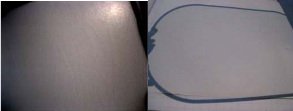
Figure 3a and 3b shadowgraphs of old (left) and new (right) ALON material.
