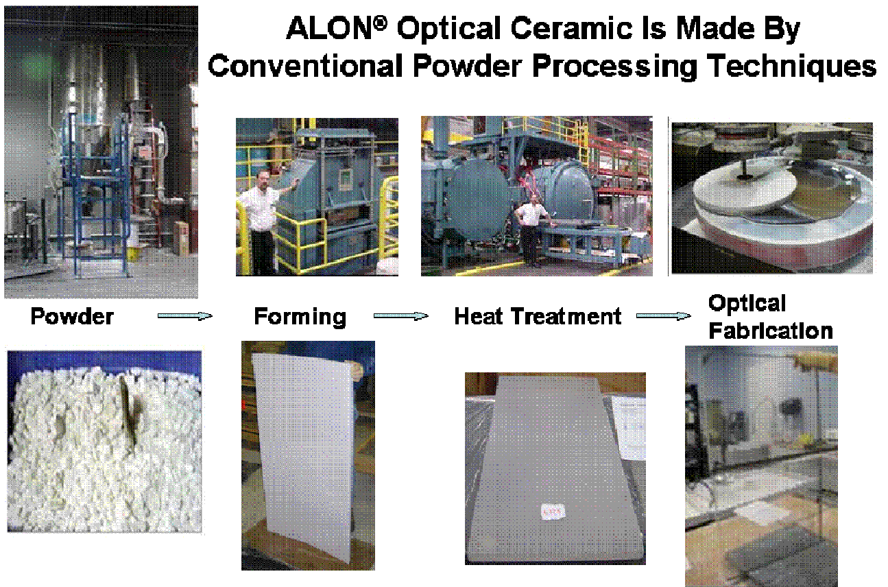
Figure 7: Schematic of process for producing ALON by powder processing
