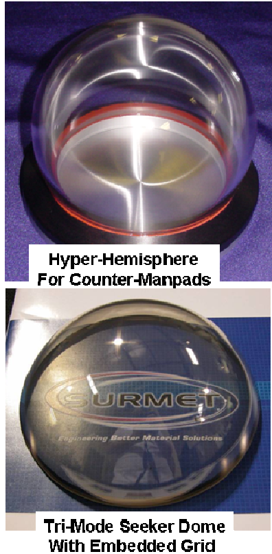
Figure 7: Photographs of a variety of ALON domes, including a hyper-hemispherical dome, Tangent ogive domes and a hemispherical dome with embedded grids.
