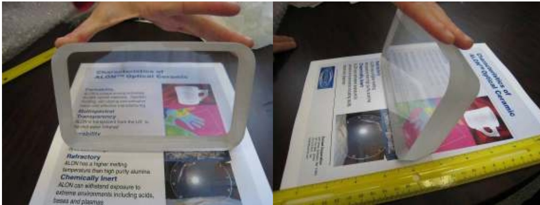
Figure 8 photograph of 1.3-in thick ALON window from the front and side.
