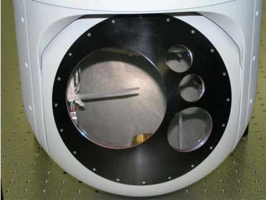
Figure 9: photograph of an ITT FALCON terminal with a window assembly with ALON® windows.
